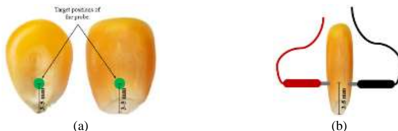
Figure 4. Probes' positions (a) on the corn seed's surface and (b) at side view
