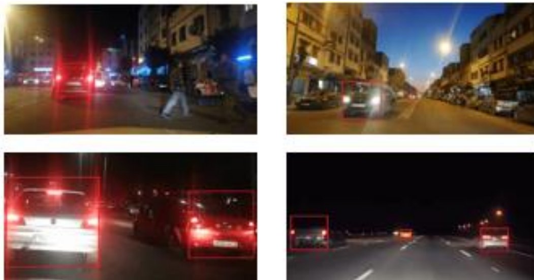
Figure 8. Some results of night-time vehicle detection
