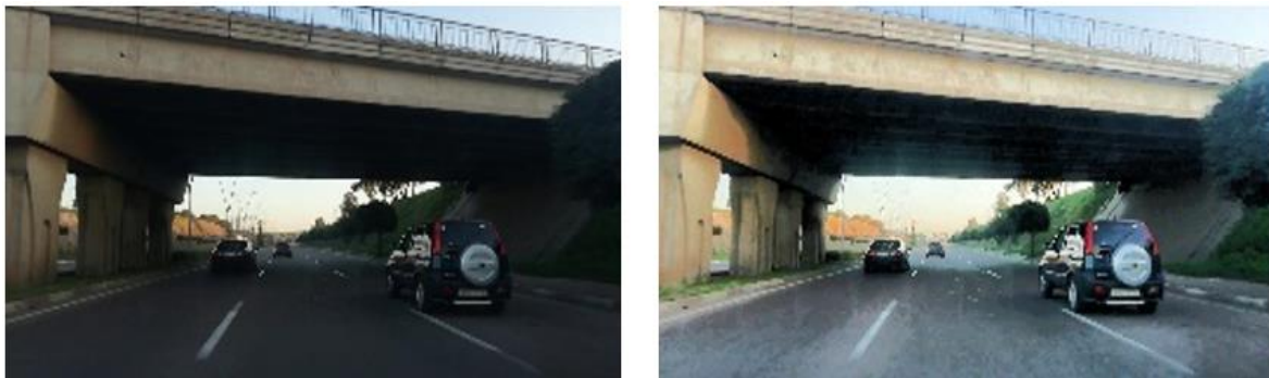
Figure 4. Image resulted after applying histogram equalization
