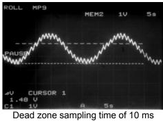
Figure 9. (a) Pulse width modulation signal to activate solenoid valve, (b). Approximation of the reference signal with triangular signal as controlled signal of ON-OFF controller
