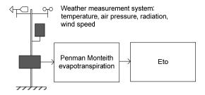
Figure 1. Schematic Diagram of Measurement of Weather Data to Calculate Reference Evapotranspiration (ET<sub>0</sub>)
