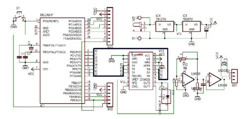
Figure 4. Electronic Architecture of Voltage Sinusiodal Signal Assumed as Input Parameters
