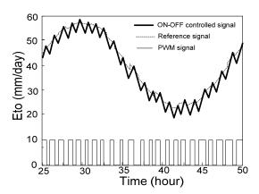
Figure 7. Performance of ON-OFF Controller (reference signal is blue, controlled signal is red, and ON-OFF condition of solenoid valve is black) with Dead Zone Sampling Time of 0.005 second [25]
