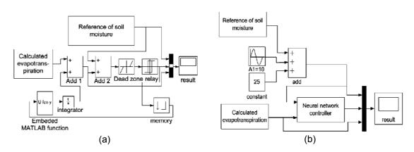
Figure 3. (a) ON-OFF controller, (b) ANN controller
