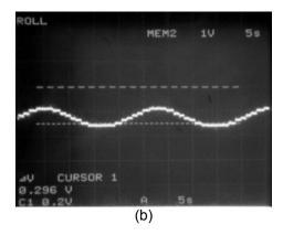
Figure 8. Oscilloscope Display of (a) Reference signal as Gaussian sinusiodal, (b) Eto signal
