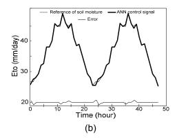
Figure 10. Error of ANN Controlled Signal Resulted by Modifying Network Architecture, (a) 1 input layer with 15 neurons and 2 hidden layers with 10 and 5 neurons and 1 output layer, (b) 1 input layer, 2 hidden layers with 96 and 1 neurons and 1 output layer
