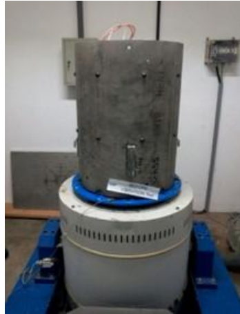
Figure 6. Payload mounted in vibration test machine
