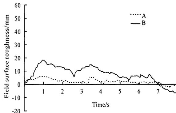
A. Field surface roughness after the compaction; B. The original field surface roughness
