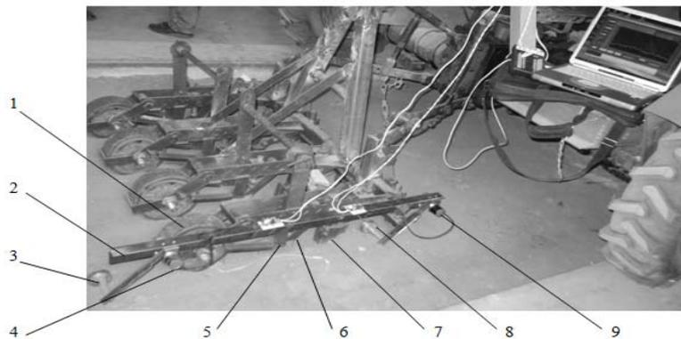
1. Compaction wheels 2. Bracket 3. Field surface roughness testing device after the compaction
