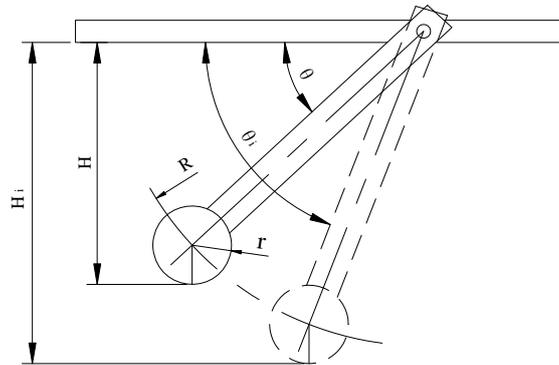
Figure 3. Schematic Diagram of the Surface Height Changes
