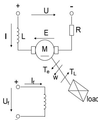
Figure 1. DC Motor Circuit and Mechanical Connection Schematic
