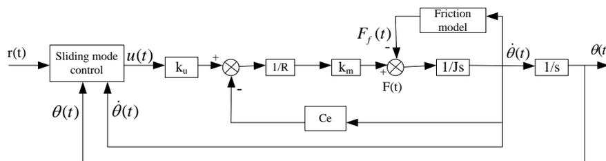
Figure 2. Control Structure Diagram of Single Shaft System
