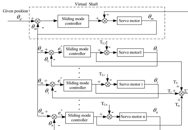
Figure 3. Structure Diagram of Electronic Virtual Line Shafting Control-Based Multi-shaft Coordinating Control System
