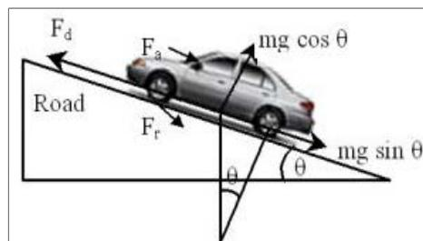
Figure 2. Forces Acting on Vehicle
