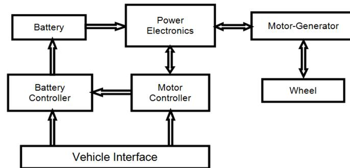
Figure 1. Electric Vehicle Drive Train with vehicle interface
