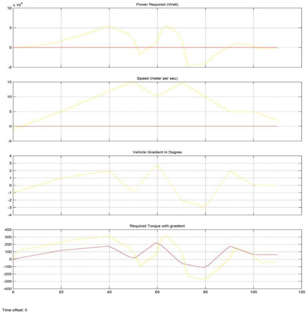
Figure 9. Vehicle Linear Speed, Gradient, Torque and Power
