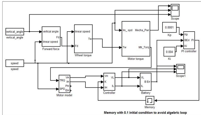
Figure 6. Forward Force Model and Motor Drive System
