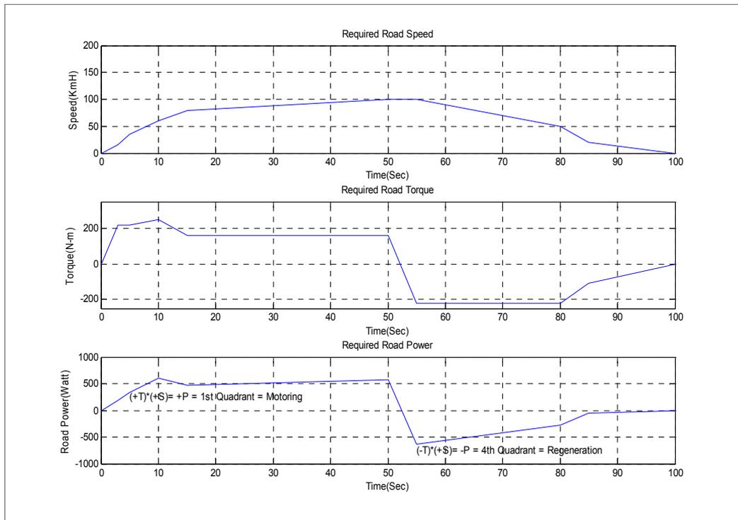
Figure 7. Road speed, Torque and Power Curves Showing Motoring and Regeneration
