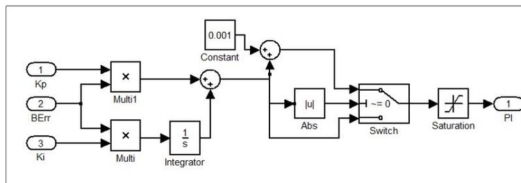
Figure 5. PI Controller Model Block
