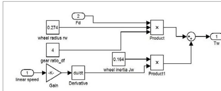
Figure 4. Wheel Torque Model Block
