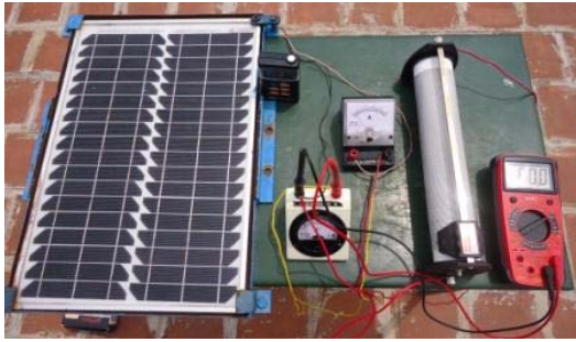
Figure 10. Experimental Setup to Find Panel VI Characteristics
