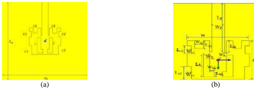
Figure 2. Distribution of slots on the patch (a) patch and slots layout of the designed microstrip antenna and (b) antenna slots with dimensional representation
