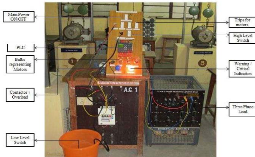
Figure 10. Hardware Model of Automation of Induction Motors
