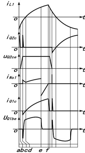
Figure 2. Key Waveforms of Conventional Self-exciting Electronic Ballast
