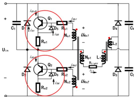
Figure 4. Ballast Schematic Diagram of Novel Circuit
