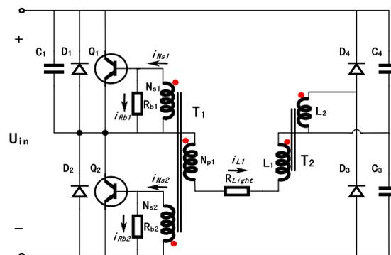
Figure 1. Schematic Diagram of Conventional Self-exciting Electronic Ballast
