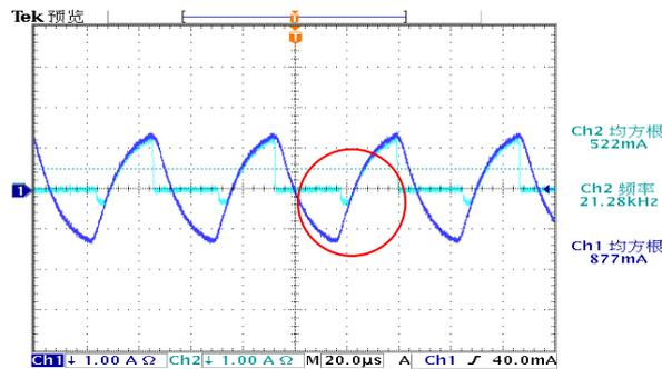
Figure 11. Current of Transistor's Current and Tank Current
