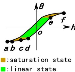
Figure 6. Track of the Magnetic T1 of Novel Circuit
