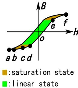
Figure 3. Track of the Magnetic T1 of Conventional Self-exciting Electronic Ballast
