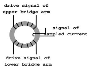
Figure 13. Wind Diagram of Single-toroid
