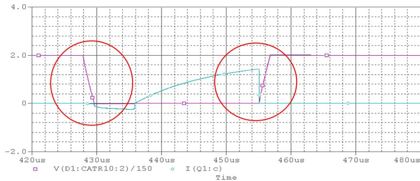
Figure 10. Switching Waveform of Transistor Q1
