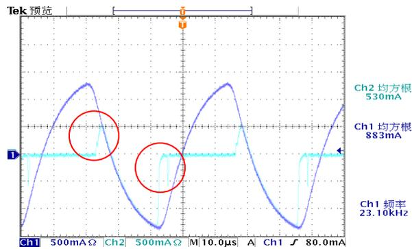
Figure 8. Current of Transistor's Current and Tank Current
