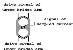
Figure 15. Wind Diagram of Balun-toroid
