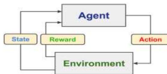
Figure 5. General structure of reinforcement learning control algorithm
