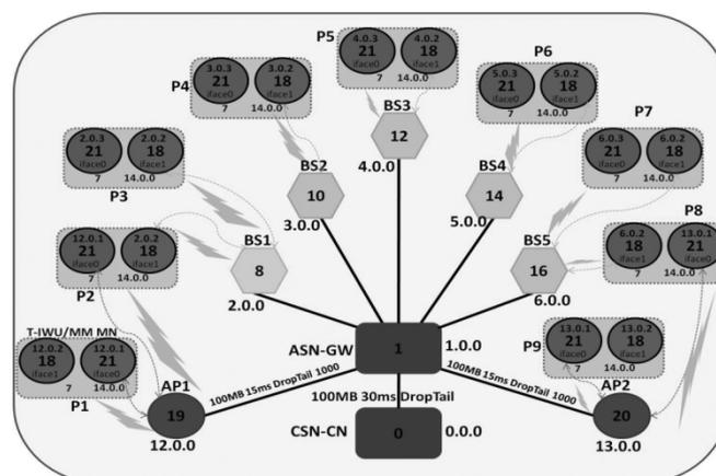
Figure 7. CoA IP Addresses Change in Heterogeneous Handover
