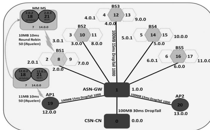
Figure 6. Heterogeneous Handover with Node ID and IP Addressing
