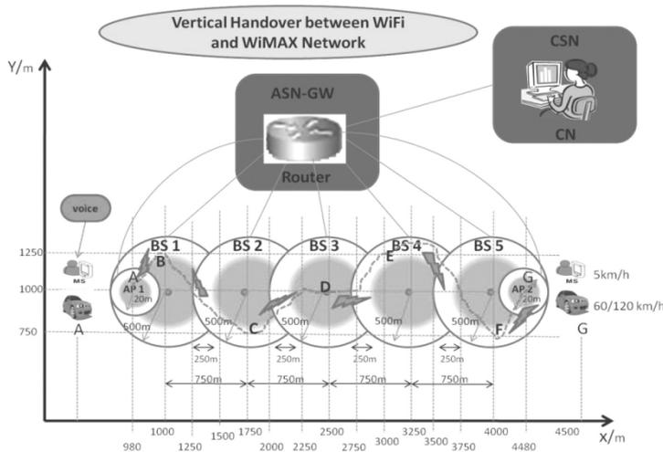
Figure 2. Heterogeneous Handover Scenario at Half-cell Overlap Coverage
