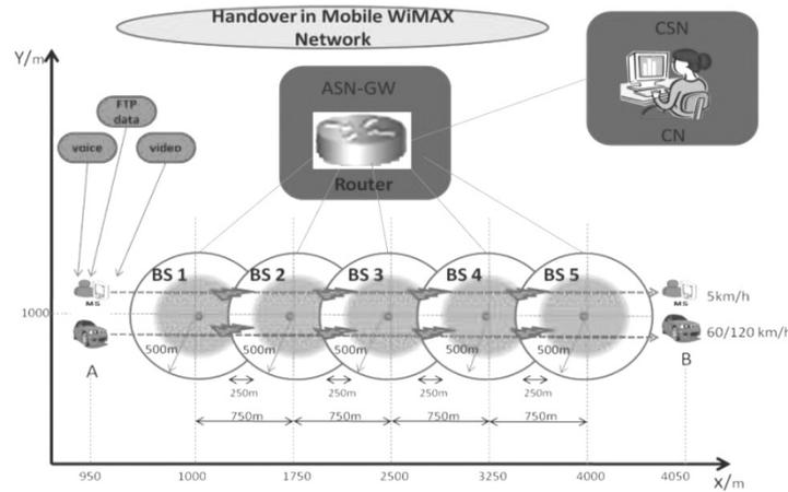
Figure 1. Homogeneous Handover Scenario at Half-cell Overlap Coverage
