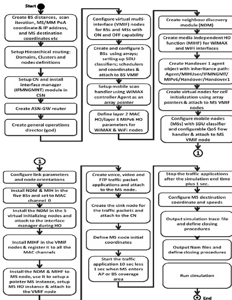
Figure 4. Simulation Flow Chart
