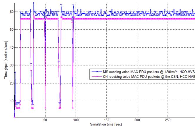
Figure 12. Throughput for High Vehicular Speed at Half-cell Overlap Coverage
