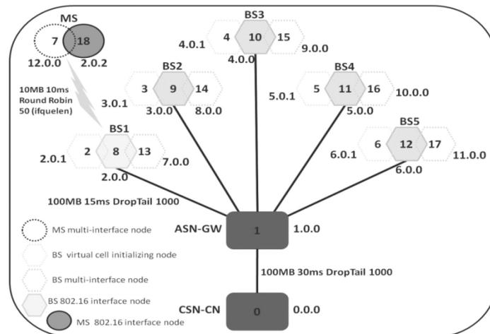
Figure 5. Horizontal Handover with Node ID and IP Addressing
