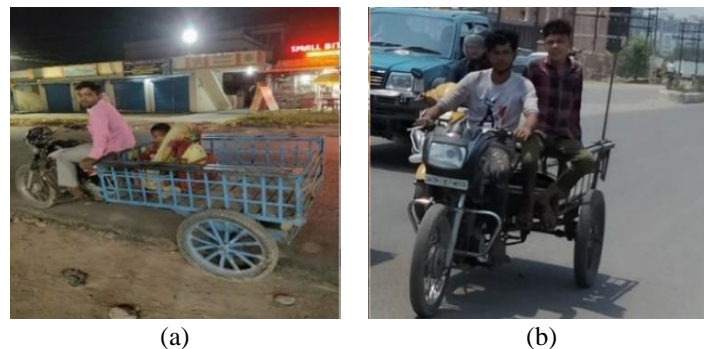
Figure 2. Displays the modified automobiles that are difficult to recognize, as seen in the images; (a) and (b) illustrate examples of modified vehicles by attaching the carrier to the motorcycle, transformed into a cargo or transit vehicle
