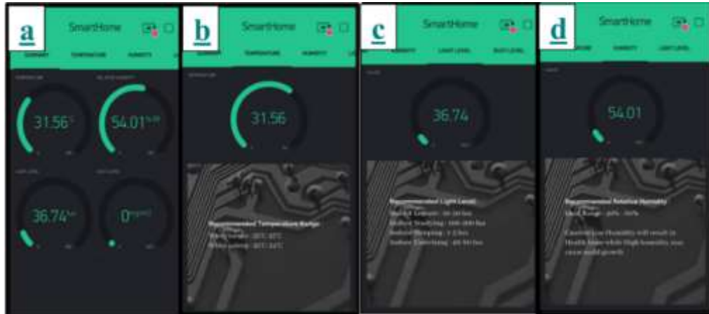
Figure 8. The customized user application involves the: (a) summary page, (b) temperature, (c) light level, and (d) %RH readings
