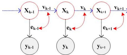
Figure 2. Process and Measurement Noise Correlation Diagram
