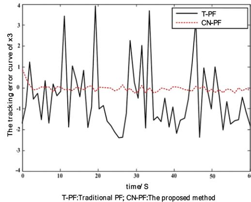
Figure 7. The Tracking Error Curve of  $x_3$
