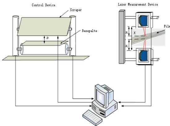
Figure 1. Film of Lithium Battery Detection
