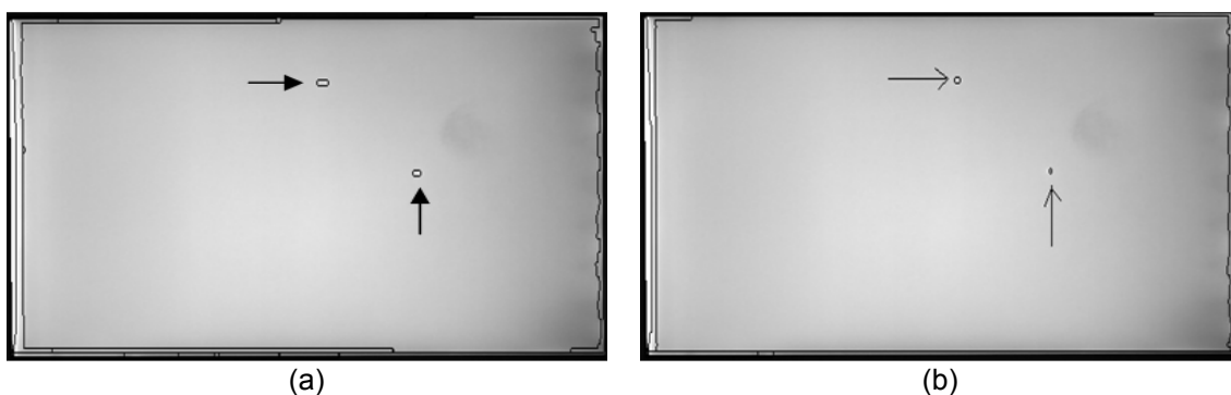
Figure 6. Defect Detection by Region Growing at Tolerance (a) 3 level, (b) 2 level
