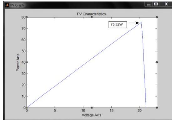
Figure 4. PV Graph Characteristics of Solar Cell
