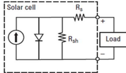
Figure 1. DC Equivalent Model of Solar Cell
