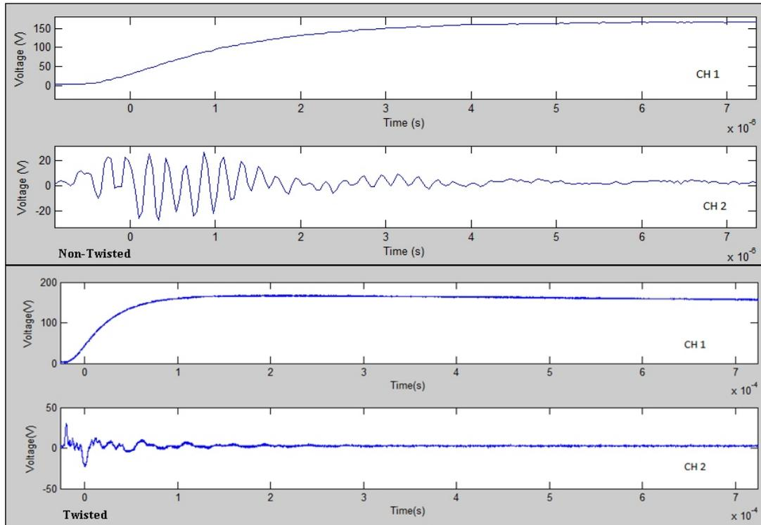
Figure 1. Profile of input signal (1.2/50  $\mu$ s) of distribution line with the peak voltage of 66 kV and the unwanted signal of solar panel at distant of 1.0 m
