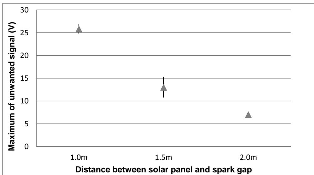
Figure 3. Gap Distance of Solar Panel and Spark Gap versus Maximum Voltage of Unwanted Signal
