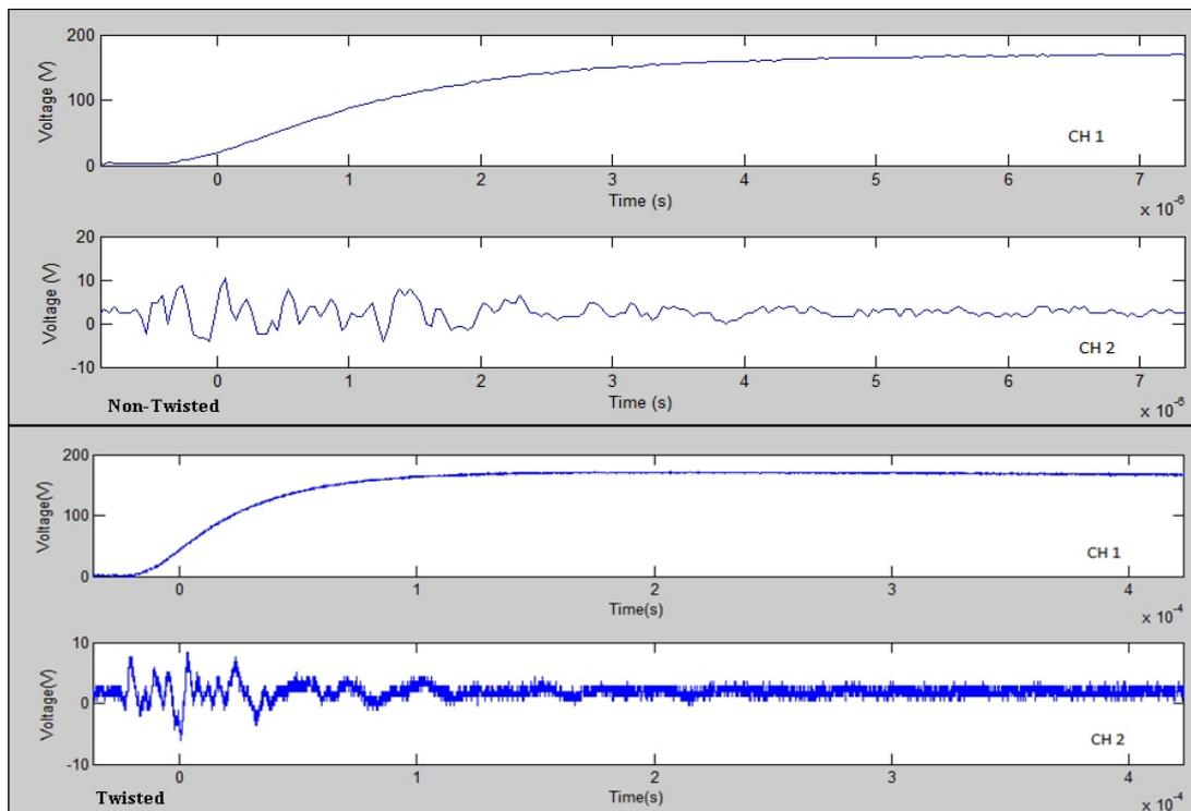
Figure 2. Profile of input signal (1.2/50  $\mu$ s) of distribution line with the peak voltage of 66 kV and the unwanted signal of solar panel of 2.0 m
