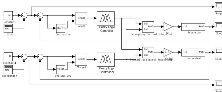
Figure 4. Simulation Model of the System
