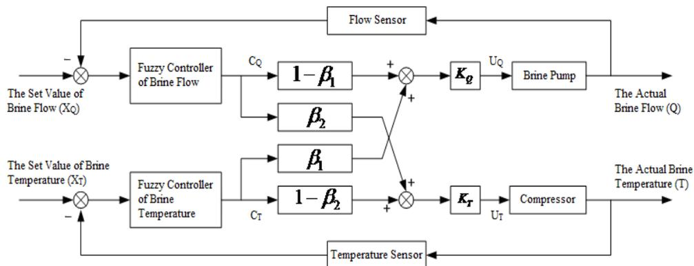
Figure 3. The System Structure of Fuzzy Decoupling Controller
