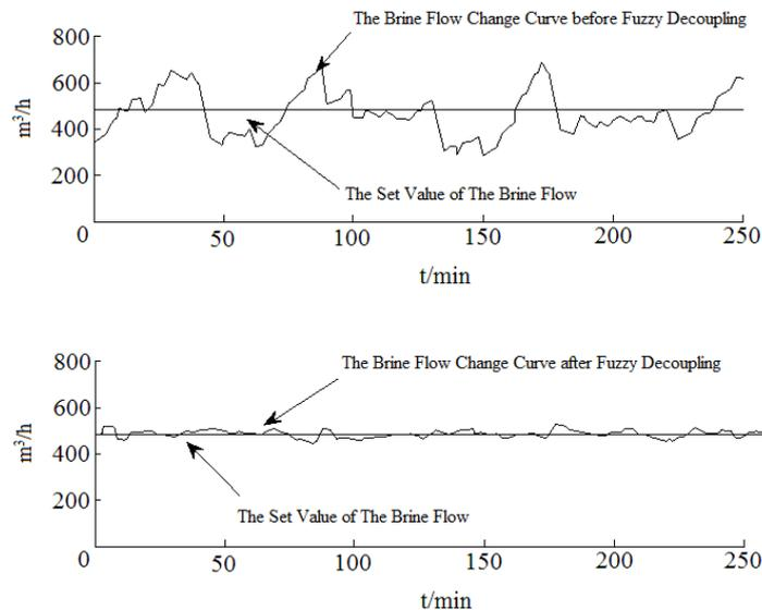
Figure 5. The Change Curve of the Brine Flow Before and After the Fuzzy Decoupling Control
