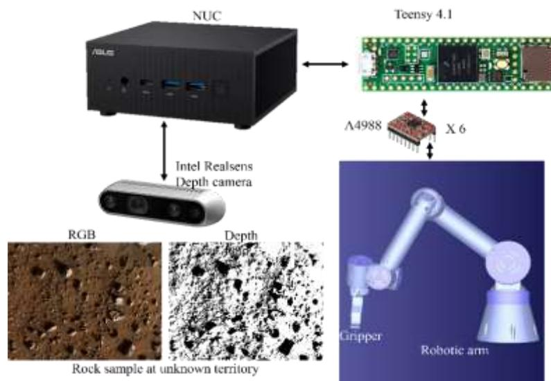
Figure 1. Proposed system diagram for the ARCAxUT
