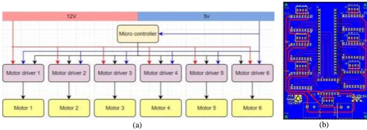
Figure 2. Circuit details for driving the motors using microcontrollers (a) block diagram showing motor interfacing with Teensy 4.1 (motor controller) and A4988 (motor driver) and (b) PCB design for Teensy 4.1 integration with NEMA 17 stepper motors
