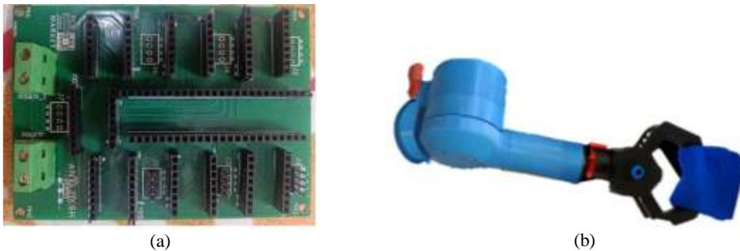
Figure 5. The circuit details and gripper assembly (a) screenshot PCB of the project after soldering and (b) image of gripper lifting the object
