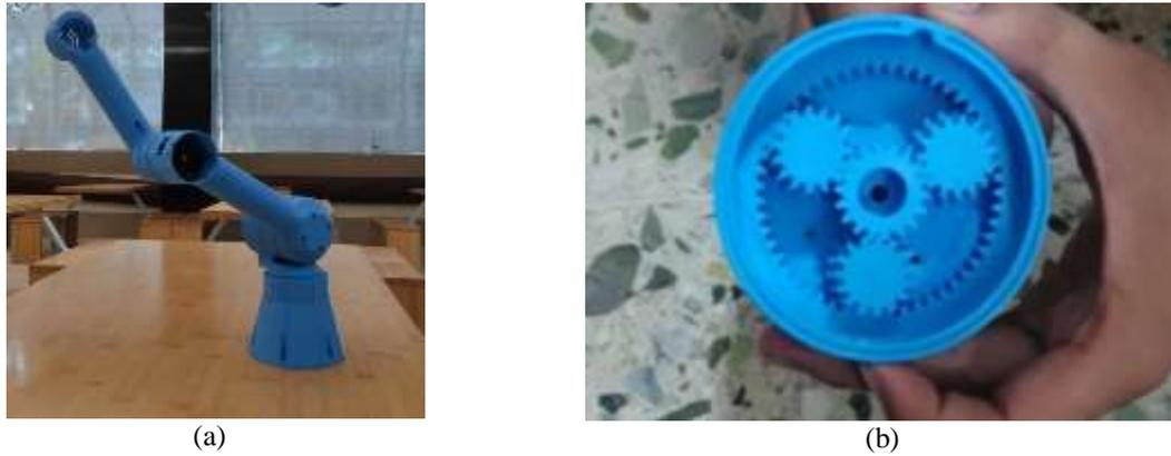
Figure 4. 3D-printed robotic arm assembly (a) picture of the 3D-printed assembly and (b) picture of internal gear mechanism
