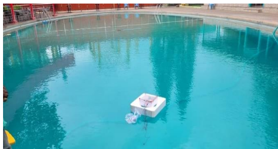
Figure 4. An energy harvester is placed in the water tank
