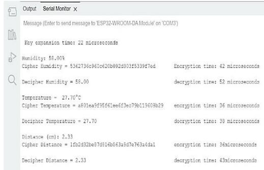
Figure 3. Output on Arduino serial for the standard S-box with ten rounds
