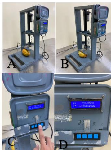
Figure 2. Process flow of compression testing: A) positioning of pod to the compression machine, B) start of pod breaking, C) end of compression test, D) reading of result
