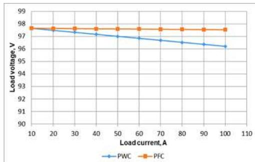
Figure 12. Output characteristics of pulse converters at rated operating conditions
