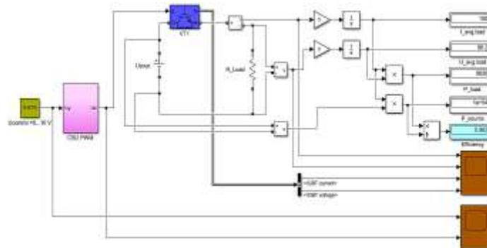
Figure 2. The model of the PWM converter
