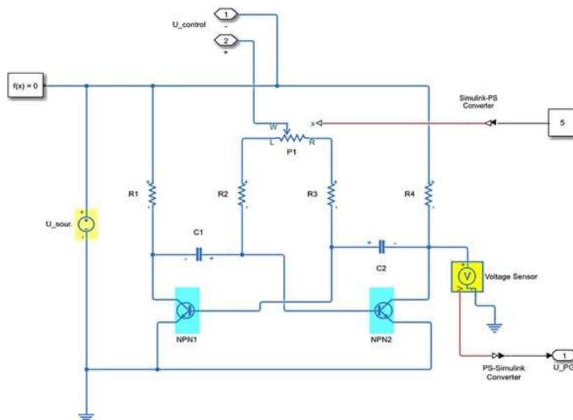
Figure 7. Square wave generator model
