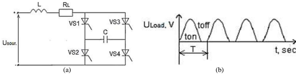
Figure 4. PFC output voltage (a) power circuit frequency-pulse converter and (b) load voltage diagrams at R-load
