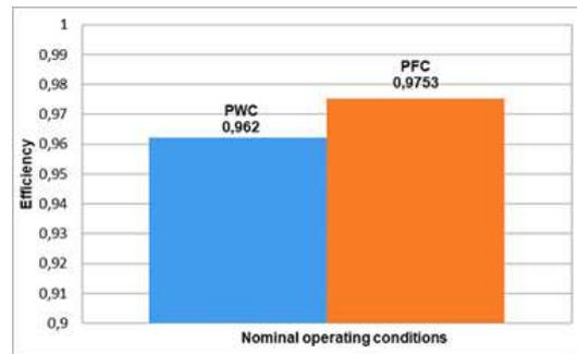
Figure 13. Efficiency of pulse converters at nominal operating conditions
