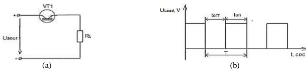
Figure 1. Basic PWM circuit (a) pulse-width modulated semiconductor converter and (b) load voltage diagrams at r-load
