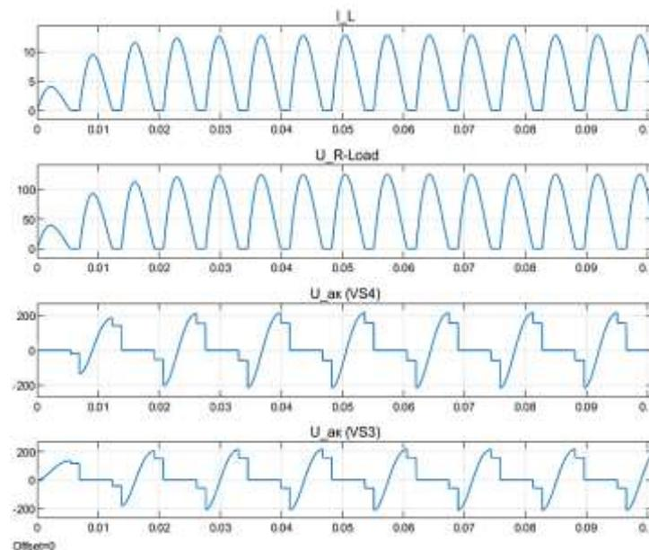
Figure 11. Dynamic characteristics of the PFC operation at a frequency of  $f = 145 \text{ Hz}$  ( $\gamma = 0.6$ ): the first graph- load current (IL); the second graph- load voltage (UR); the third graph- voltage (Uak) of the thyristor VS4; the fourth graph - voltage (Uac) of the thyristor VS3
