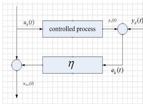
Figure 2. The Structure and Process of ILC Control Method
