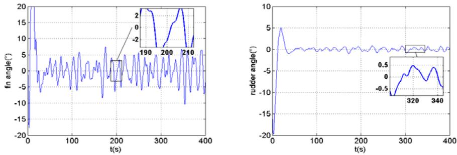
Figure 2. Fin Angle and Rudder Angle under Grade 6 Wave
