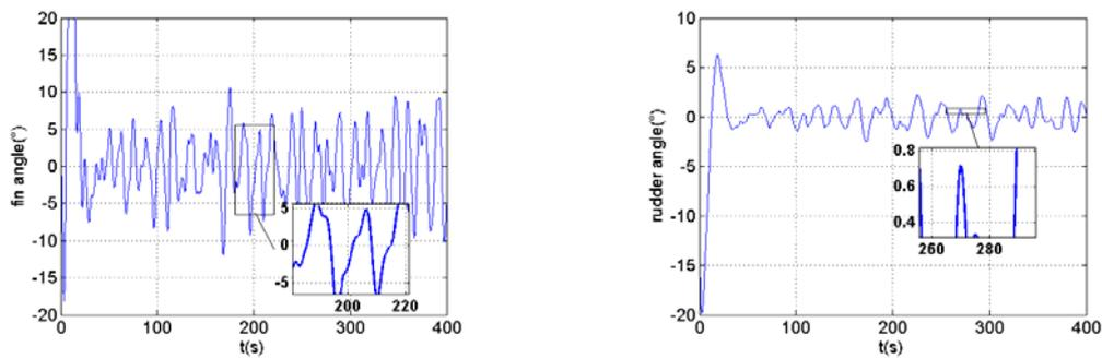
Figure 4. Fin Angle and Rudder Angle under Grade 8 Wave
