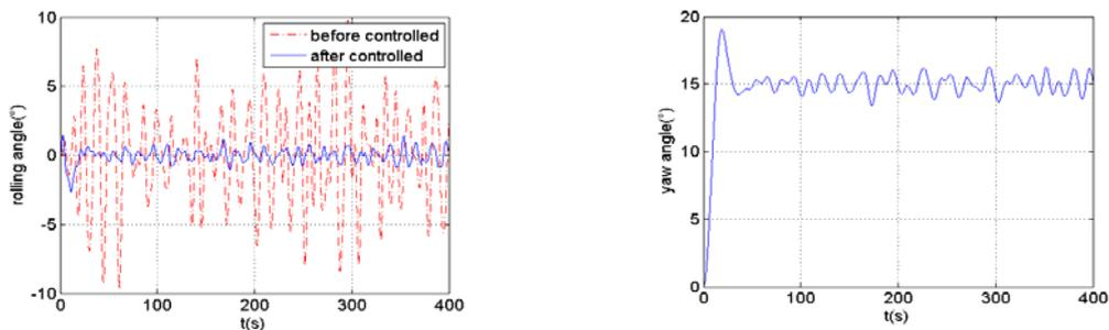
Figure 3. Rolling Angle and Yaw Angle under Grade 8 Wave
