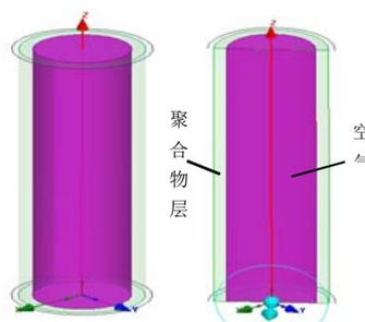
Figure 2. The HFSS Model (left) and Positive Section (right) for the THzTeflon Tube
