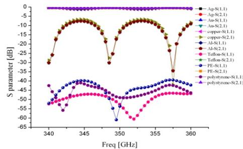
Figure 1. The S Parameters for Tube with Different Metal and Polymer Materials
