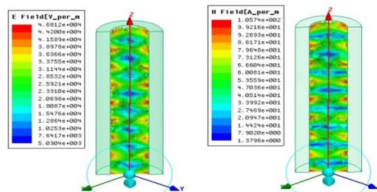
Figure 4. The Field Profile for Single Medium THz Teflon tube: Electric Field (left) and Magnetic Field (right)
