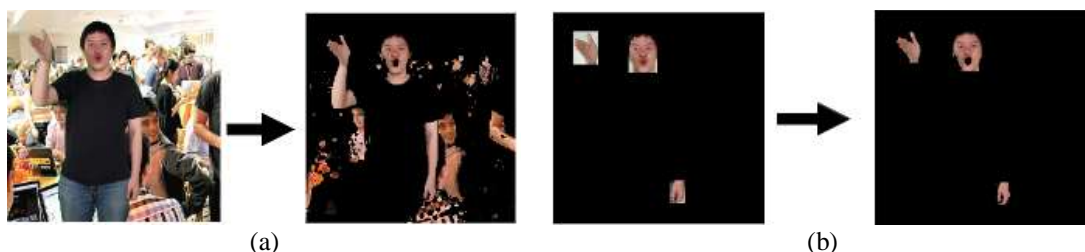
Figure 6. Comparison of segmentation results (a) without object detection and (b) with object detection
