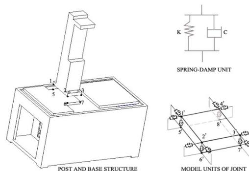
Figure 3. The Equivalent Mode of Base and Post
