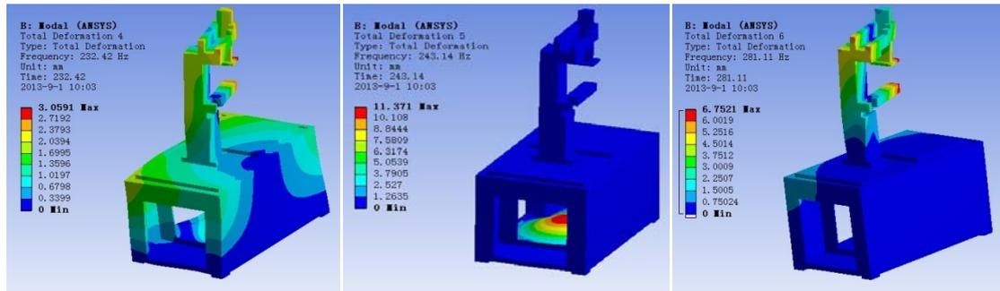
Figure 5. The Second Three Modes of the Whole Machine Tool
