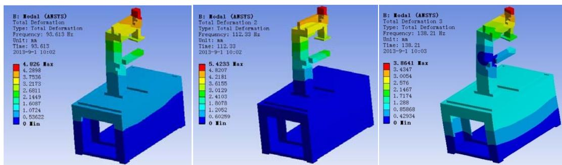
Figure 4. The First Three Modes of the Whole Machine Tool
