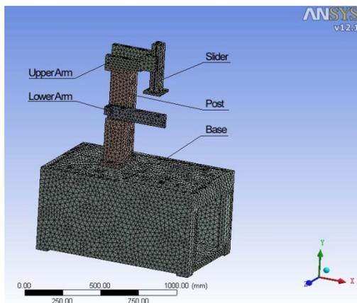
Figure 1. The Finite Element Model of Machine
