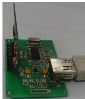
Figure 13. Zigbee Wireless Receiver Monitoring of the Test Chamber
