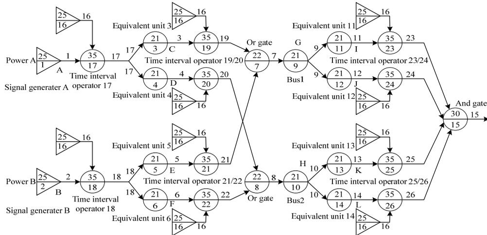
Figure 3. The Simplified GO - FLOW Chart for Traction Power Supply System
