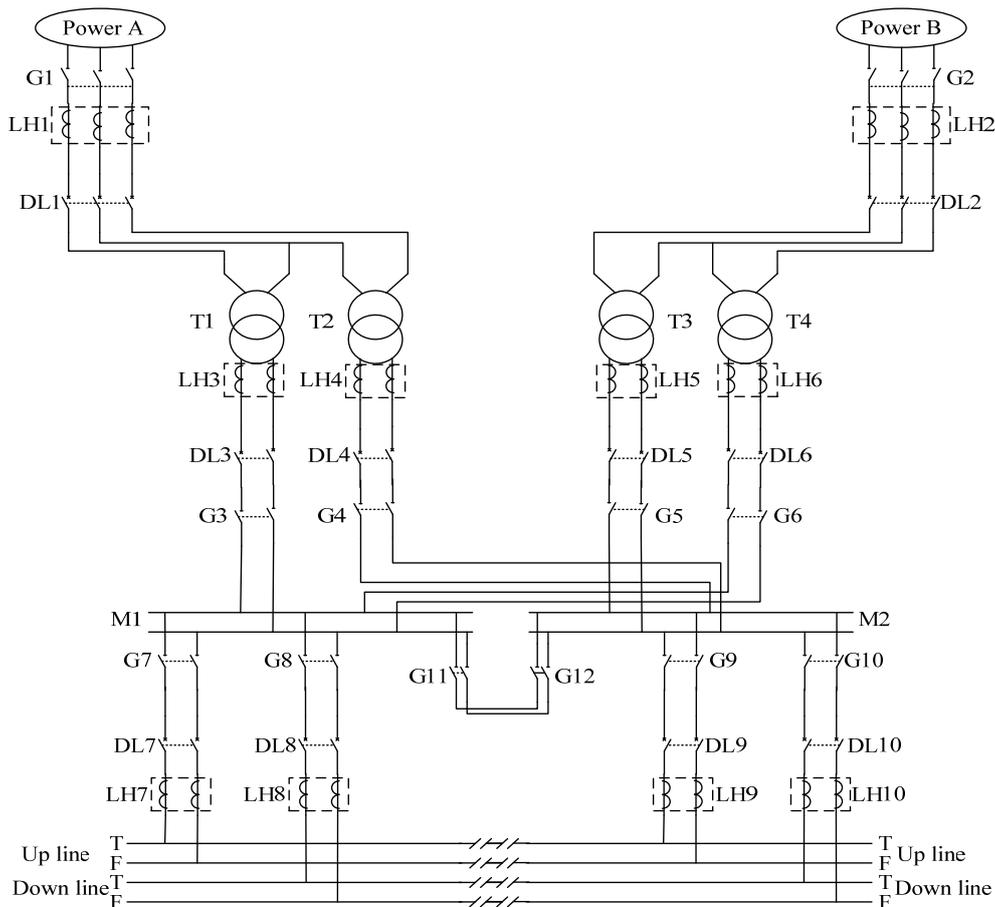
Figure 2. Schematic Diagram of Traction Power Supply System
