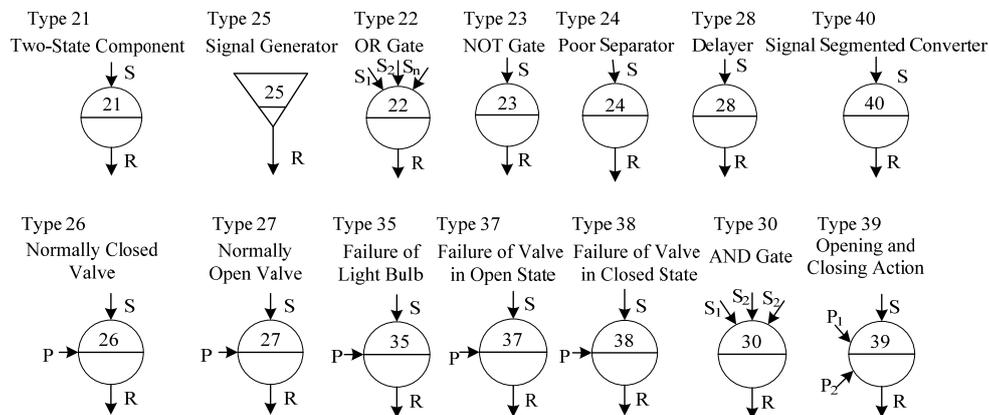
Figure 1. Operators in the GO - FLOW Methodology
