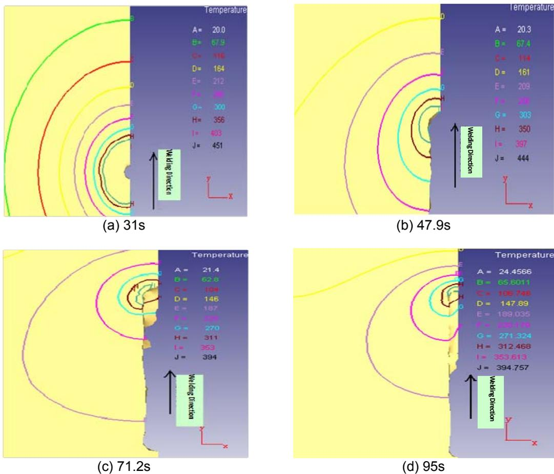
Figure 5. The isothermal Diagram on Half X-Y Section at Different Time ( °C)
