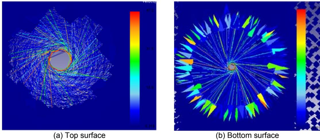
Figure 11. Flow Distribution (velocity) on Top and Bottom Surface for Workplate
