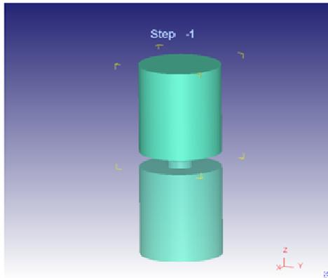
Figure 3. Bobbin Tool Geometry Model
