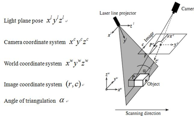
Figure 2. Sheet-of-light Vision Measurement Principle
