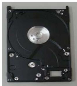
Figure 1. Measured Object: Hard-disk of Computer
