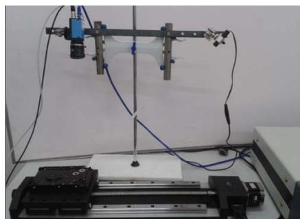
Figure 6. Real Object of Line Structured Light Vision Sensor
