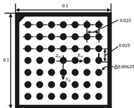
Figure 3. Calibration Board and Specific Dimensions
