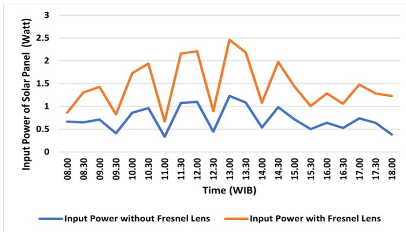
Figure 11. Output power of solar panel
