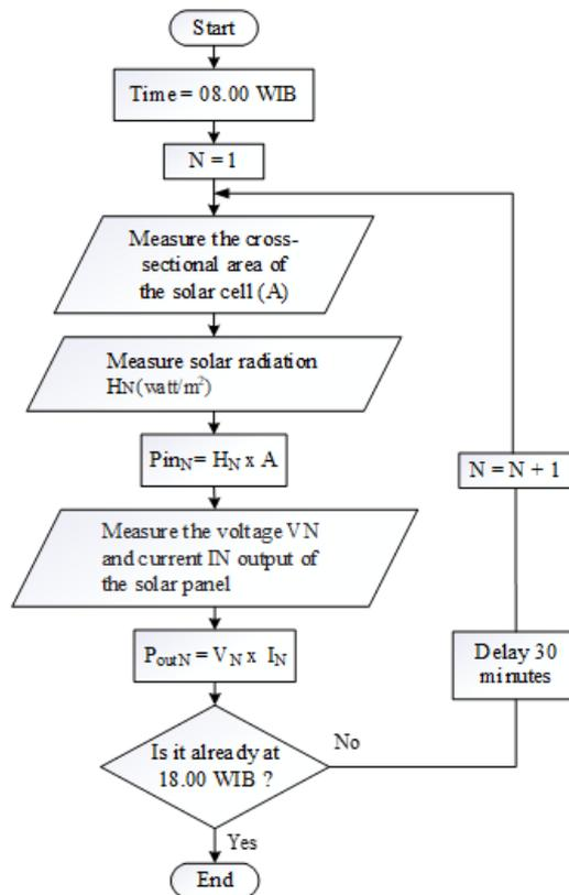
Figure 6. Flowchart diagram of solar panel output power measurement patterns
