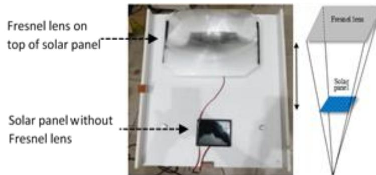
Figure 4. Position the Fresnel lens above the solar panel
