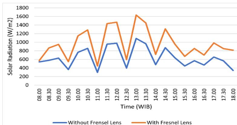
Figure 9. Solar radiation without and with a Fresnel lens
