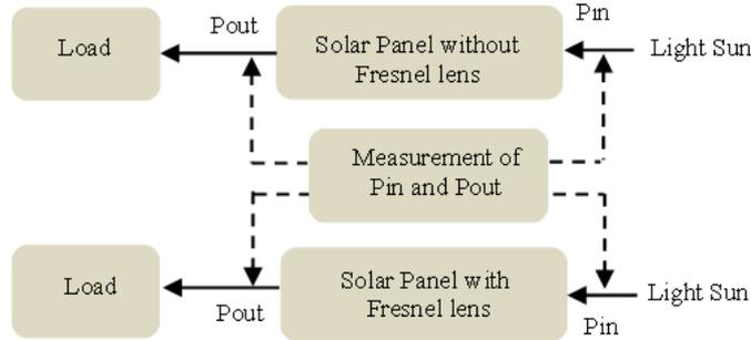
Figure 5. Block diagram of measurement pattern
