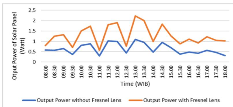
Figure 10. Graph of solar panel input power
