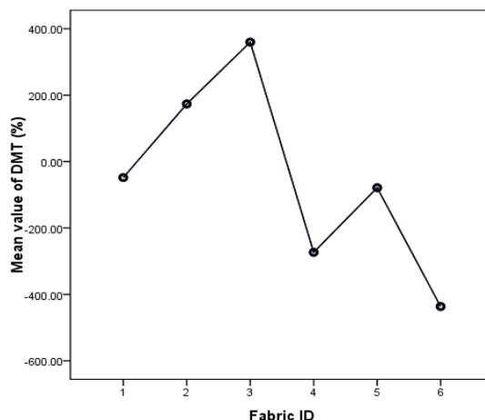
Figure 5. Mean Value of the Test Results of Moisture Transport Difference ( $D_{MT}$ )
