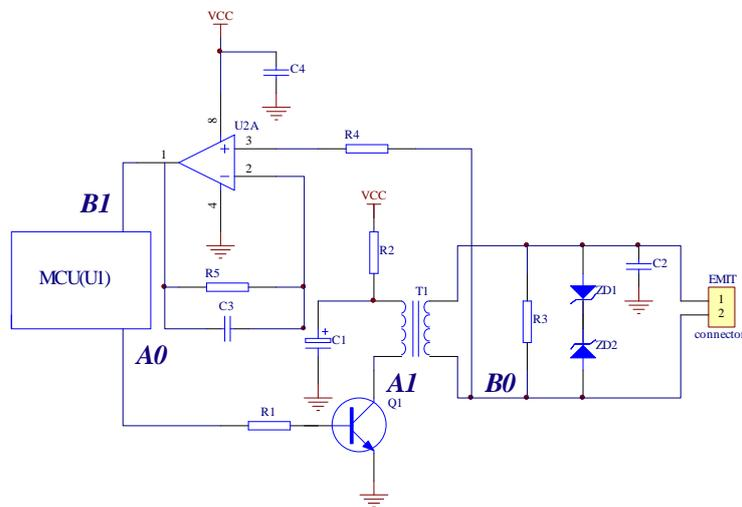
Figure 2. Sensor Signal Transceiver Schematic Diagram
