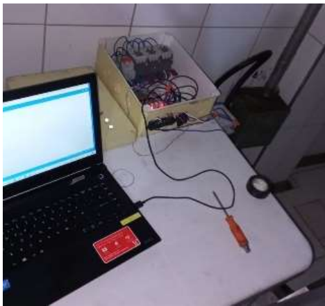
Figure 27. Physical system implemented with sensor at gas tap
