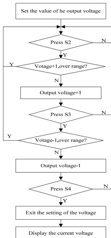
Figure 4. The Flow Chart Key Detection
