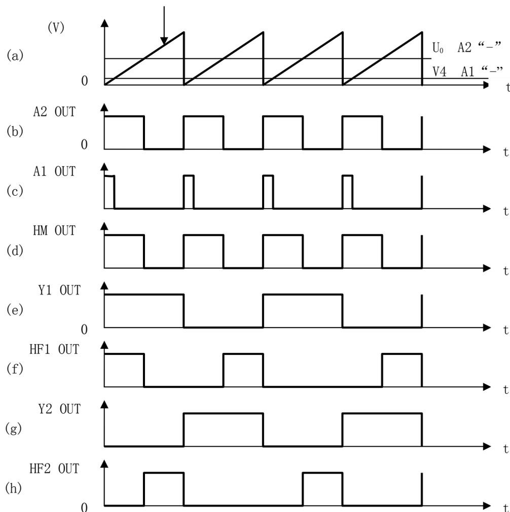
Figure 2. The Change of TL494 Output Wave
