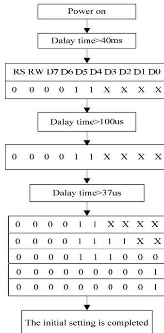
Figure 5. The Interface Program of LCD
