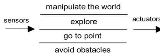
Figure 2. Behavior-base Control Architecture
