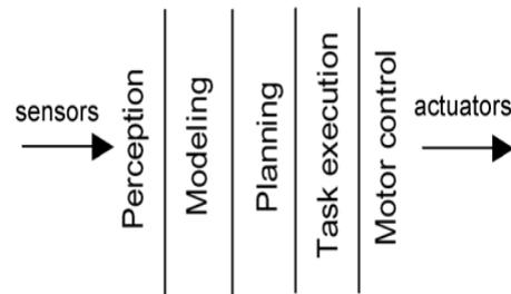
Figure 1. Phase of Traditional Control Architecture
