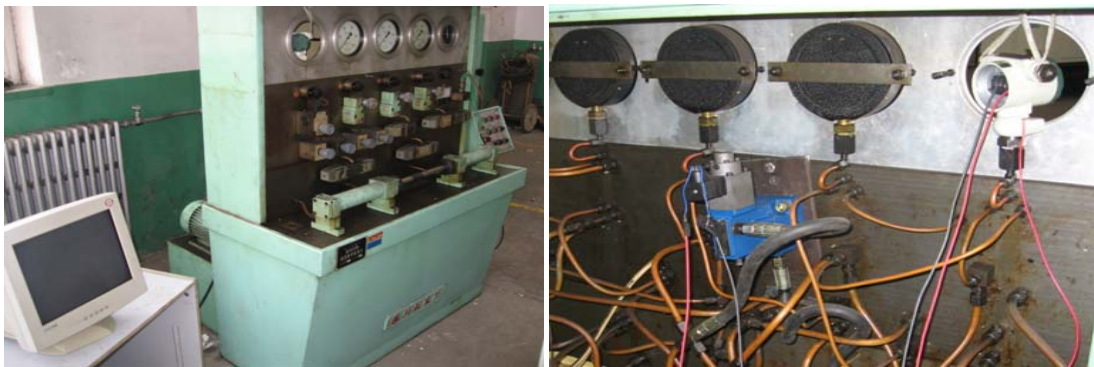
Figure 2. Reform Design Diagram of Pressure Adjustment Platform of Proportional Relief Valve
