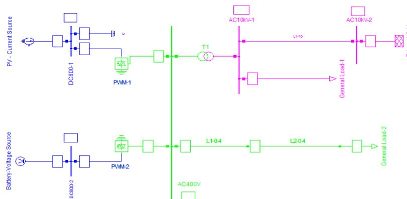
Figure 5. The Topological Diagram of Equivalent Network of Distribution Subsystem
