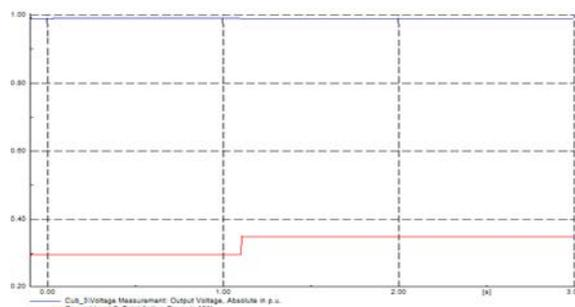
Figure 9. The Voltage Dynamic Response of Parallel Point (based 1kV)
