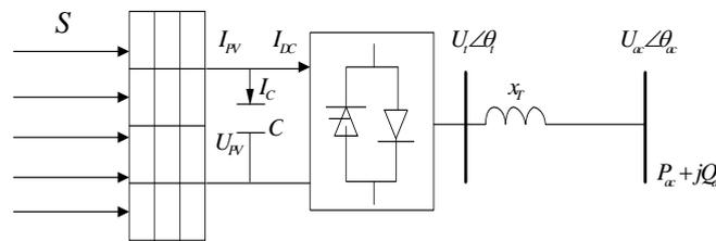
Figure 3. The Model of Photovoltaic Paralleled in System
