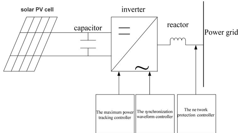
Figure 1. The Structure of Photovoltaic Paralleled in System
