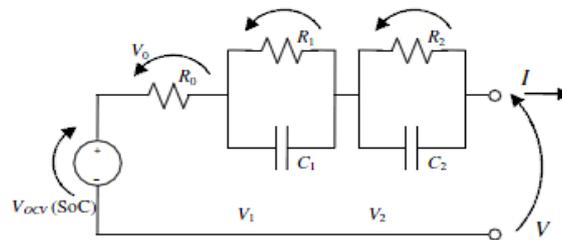
Figure 4. The Detailed Equivalent Circuit of Stored Energy Battery
