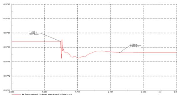
Figure 8. The Voltage Dynamic Response of Parallel Point (based 1kV)
