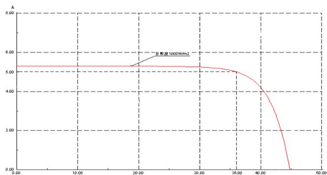
Figure 2. The Characteristic Curve of 125 Single-crystal Silicon Photovoltaic Module
