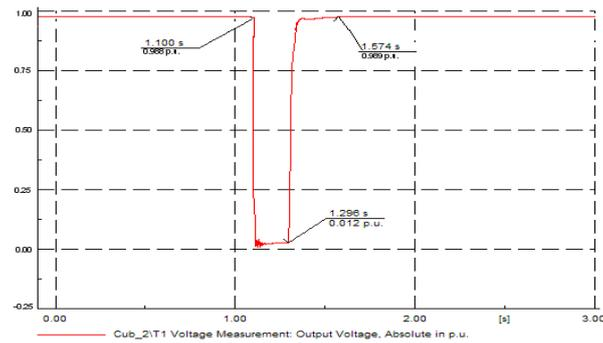
Figure 6. The Voltage Dynamic Response of Parallel Point (based 1kV)
