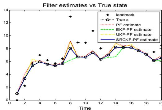
Figure 1. Results of the PF-SLAM Algorithm, the EPF-SLAM Algorithm, the UPF-SLAM Algorithm and the SRCPF-SLAM Algorithm under the Gaussian Noise
