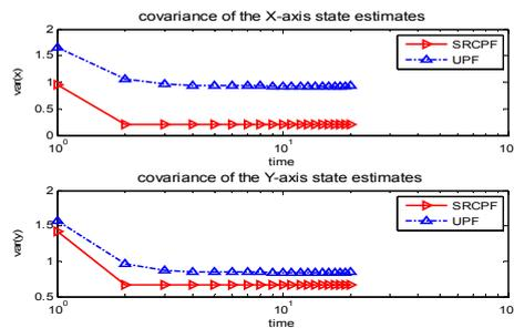
Figure 2. The State Estimates Covariance of the SRCPF Algorithm on the X, Y Coordinates of the Mobile Robot Position with the State Estimates Covariance of the Latest UPF Algorithm on the X, Y Coordinates of the Mobile Robot Position under the Gaussian Noise
