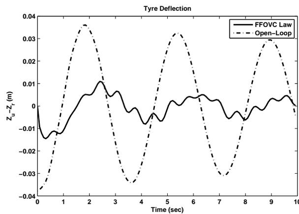
Figure 5. The curve of tire deflection
