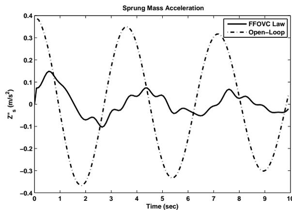
Figure 3. The curve of sprung mass acceleration
