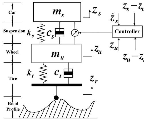
Figure 1. The two-degree-freedom quarter-car active suspension system
