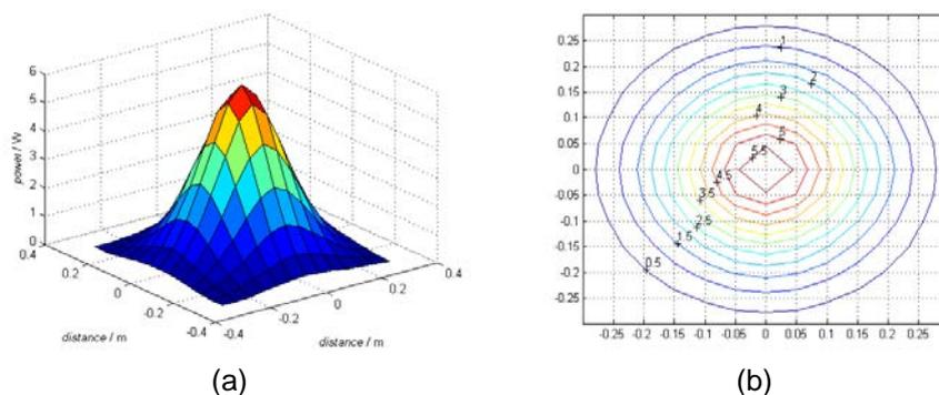
Figure 11. Received Power at 200mm Height (88KHz)
