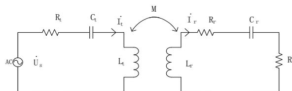
Figure 6. Simple Wireless Power Transfer System Model
