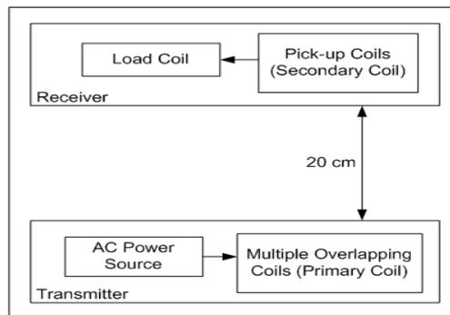
Figure 1. Wireless Power Transfer System Model
