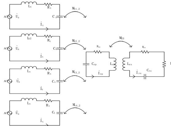
Figure 7. Wireless Power Transfer System Model for Four Coils Structure
