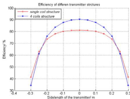
Figure 8. Comparison between Single Coil and Four Coils Structure (370KHz, 200mm Height)
