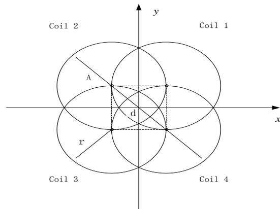
Figure 3. Four Coils Transmitter Structure
