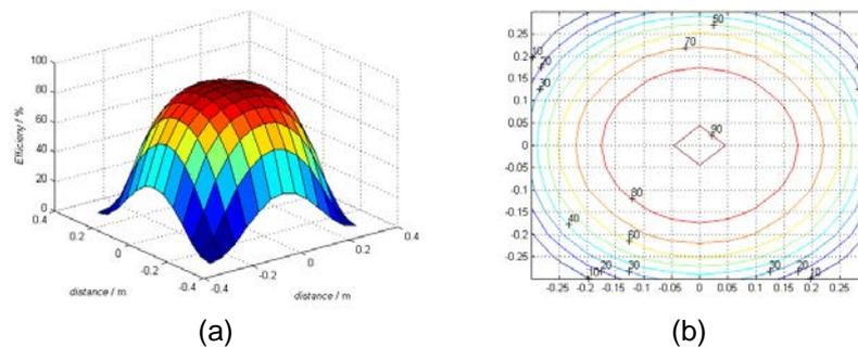
Figure 14. Power Efficiency at 200mm Height (370KHz)
