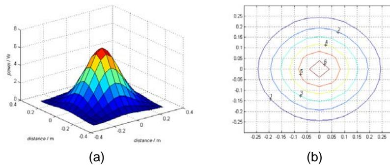
Figure 13. Received Power at 200mm Height (370KHz)
