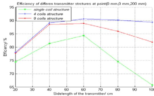
Figure 10. Received Power Efficiency for Different Transmitter Sizes
