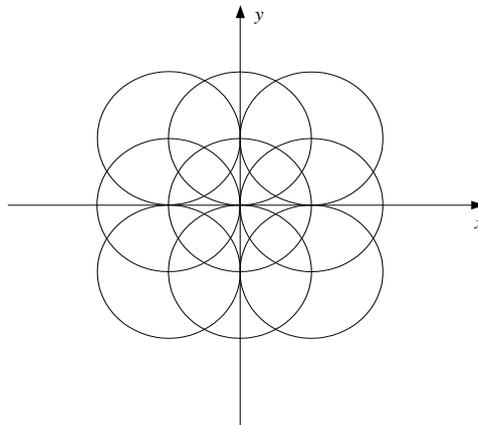
Figure 4. Nine Coils Transmitter Structure
