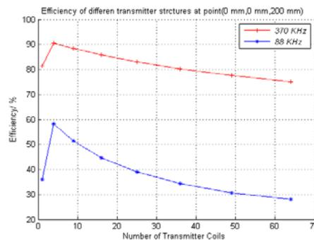
Figure 9. Received Power Efficiency for Different Multiple Coils Transmitter Structures
