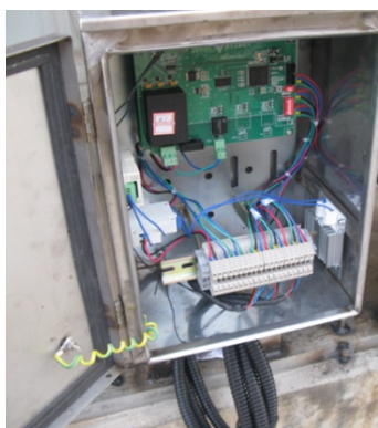
Figure 8. Structure of Terminal Device Figure 9. IED of Capacitive Equipment
