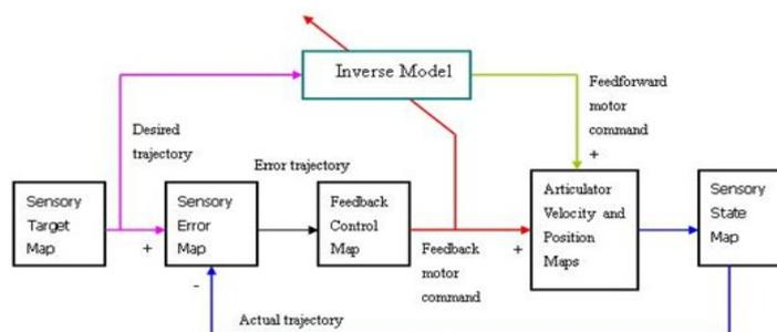
Figure 4. The Cerebellar Feedback-error Learning Model Based on DIVA Model
