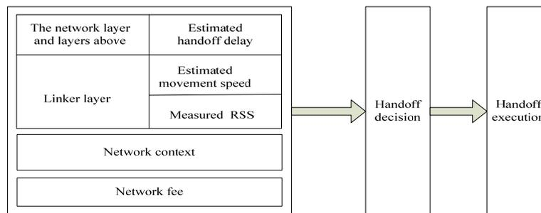
Figure 2. A Cross Layer Vertical Switch Control Model
