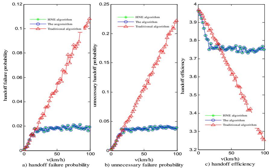
Figure 9. The Handoff Performance when MN Moves into WLAN,  $\Delta E_i \geq \ln \frac{3}{2}$
