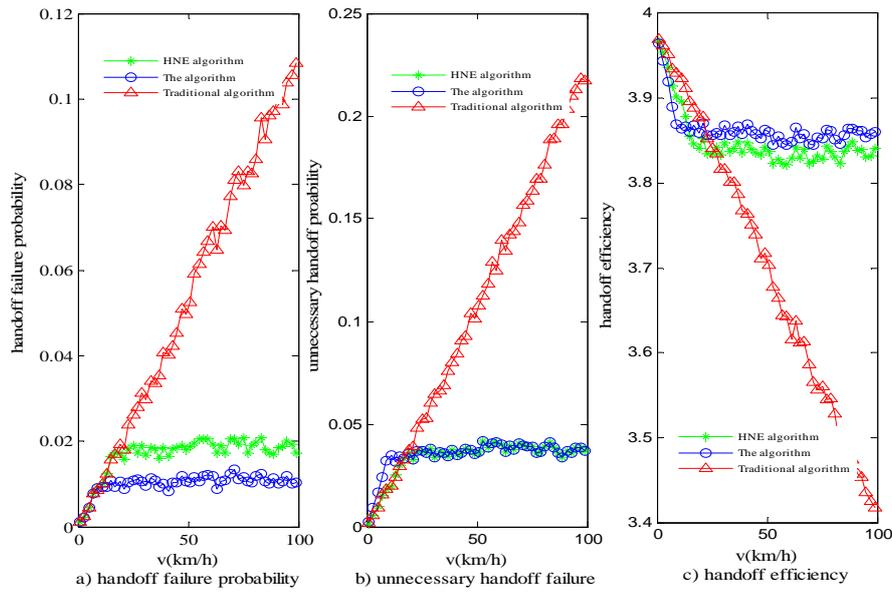
Figure 8. The Handoff Performance when MN Moves into WLAN,  $0 < \Delta E_i < \ln \frac{3}{2}$
