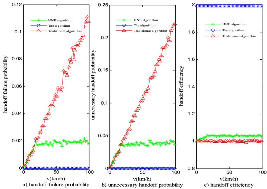
Figure 6. The Handoff Performance when MN Moves into WLAN,  $\Delta E_i < 0$
