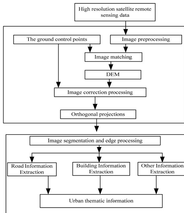
Figure 5. Satellite Remote Sensing Data Processing
